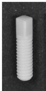
Figure 1. Experimental Zirconia implant. 1.6mm in diameter, 8mm in length.
